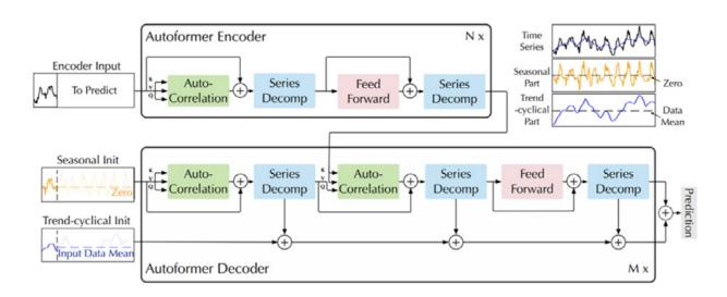
Figure 1: Autoformer architecture. The encoder eliminates the long-term trend-cyclical part by series decomposition blocks (blue blocks) and focuses on seasonal patterns modeling. The decoder accumulates the trend part extracted from hidden variables progressively. The past seasonal information from encoder is utilized by the encoder-decoder Auto-Correlation (center green block in decoder). Image source: https://huggingface.co/blog/autoformer
